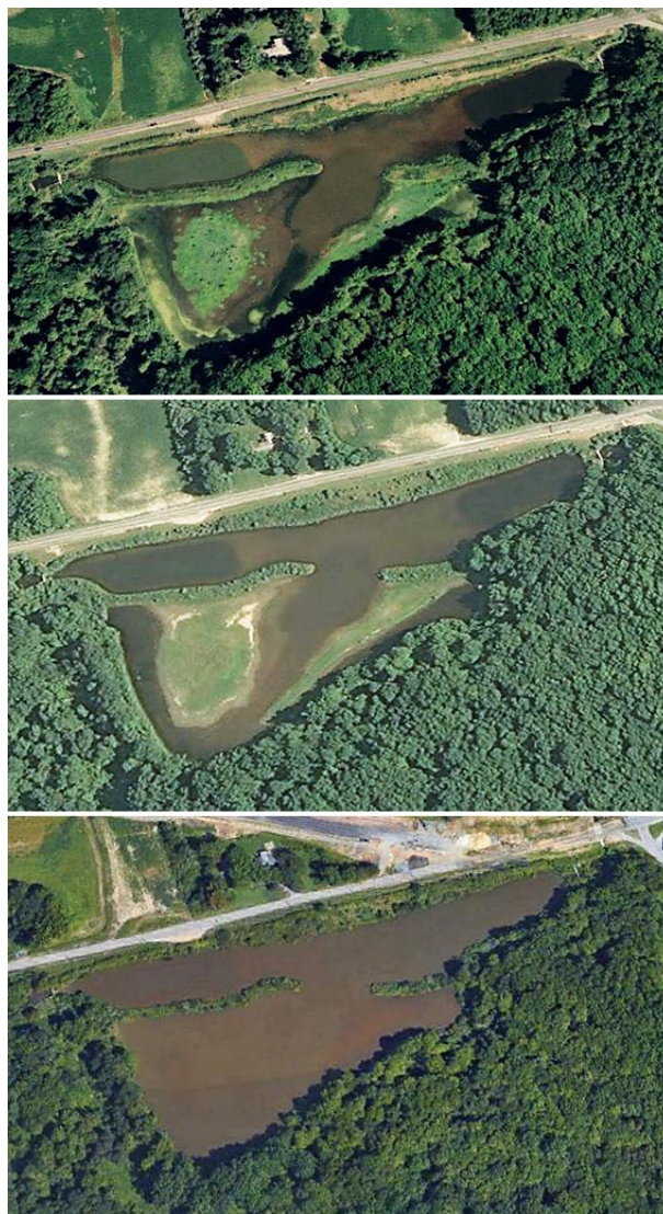
Figure 4. Three Google Earth images of the Wetland Mitigation Pond taken in 2004, 2009, and 2015, top to bottom. The color of the water surface in the earlier images corresponds to differences in depth with the greatest depth of over 10 feet in two deeper excavations, one on the eastern end and the other on the western end. The water level is higher in the most recent image due to beaver obstructing the exit gates.
